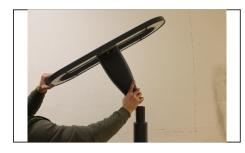
12. To change the luminaire tilt, unscrew the Allen screws, set the desired angle and screw the Allen screws back again with a tightening torque of 4-4,9 Nm.
