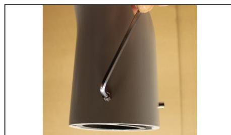
10. Take out an inner adepter from the bottom part of the luminaire. Fix the luminaire on the post. Tighten allen screws with tightening torque of 8 Nm.
